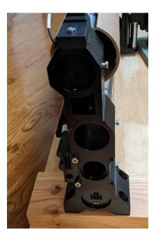
And finally the redesigned spindle mount. What was done here was to disassemble OneFinity's Z-20, then replace the round mount with a flat plane mount.
