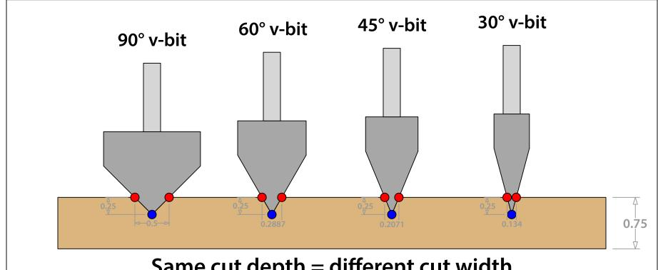
Same cut depth = different cut width (The angle of the bit determines the width of the cut.)
